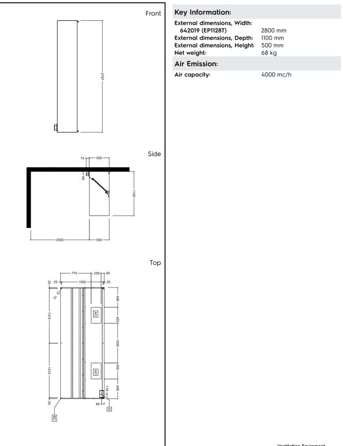
Ventilation Equipment 304 S/S Wall Hood+Filters 2800X1100mm
